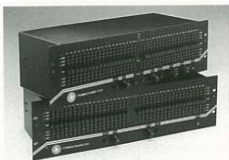
Formula Sound's first 'product line' equipment, the S19G graphic equaliser and S19GA graphic/analyser were later redesigned to become the tamper-proof SE2 series of system equalisers.
